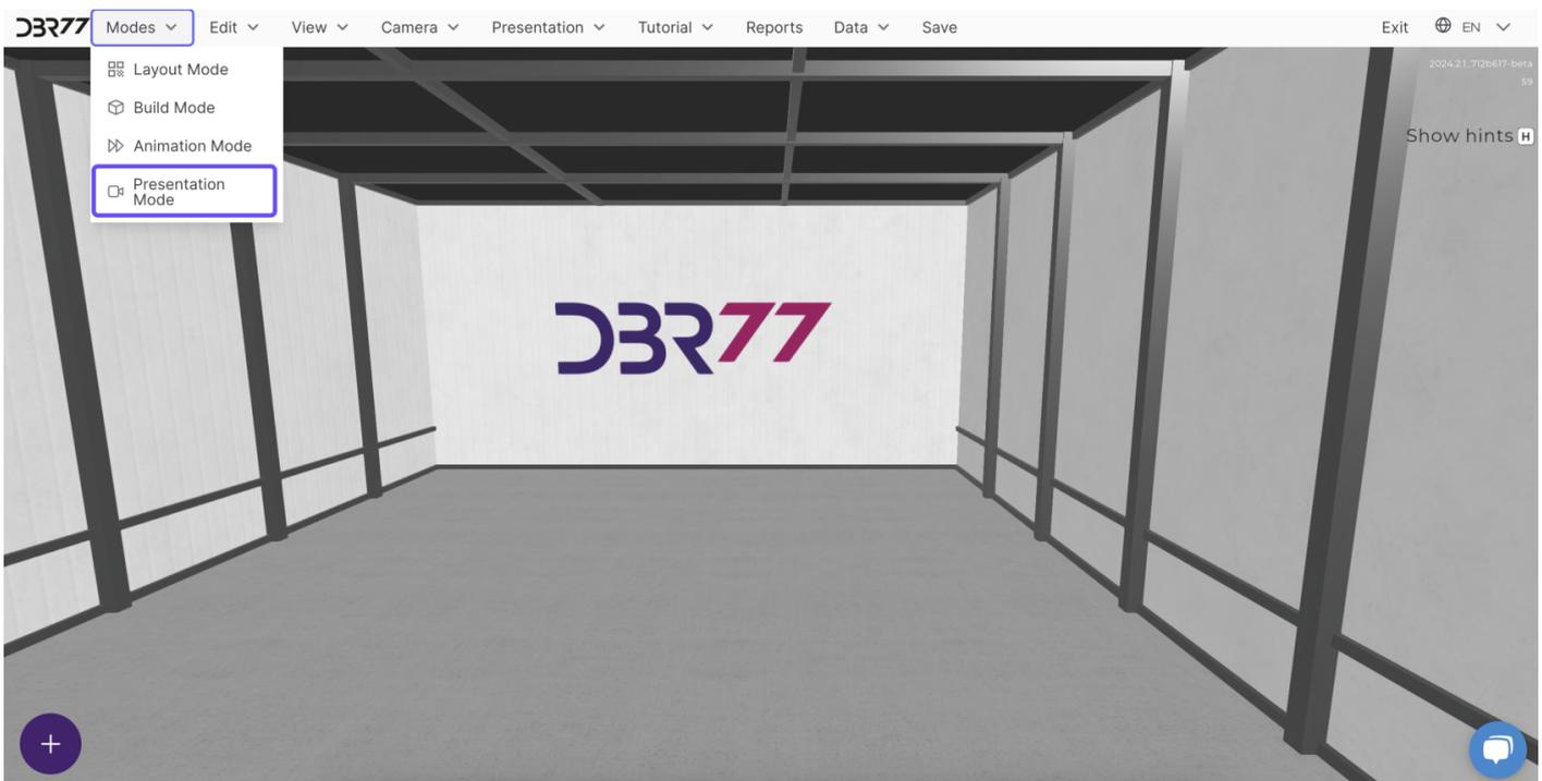
**Presentation Mode** allows you to set up desired camera perspectives for optimal visualization of operations and production processes. In this mode, you can:
